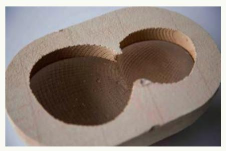
Figure 15. Cast glass in 3D printed mould.
