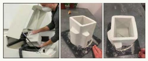
Figure 21. 3D printed moulds for glass casting, pre-firing.
