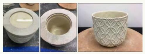
Figure 18. Slip casting porcelain using the 3D printed mould.
