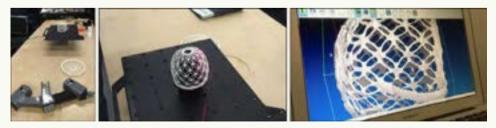
Figure 3. Polhemus Scorpion handheld 3d laser scanner; the scanning process; and the 3D scan.
