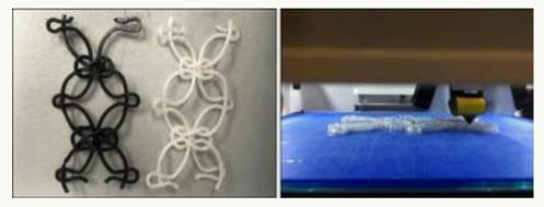
**Figure 11.** Comparison knots prints from different printers and a side view of the print process showing support material.
