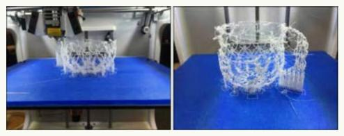
Figure 7. The first 3D printing of the cup on Tinkerine DittoPro 3D printer.
