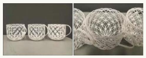
Figure 8. Printed cups in three different thicknesses: 0.8mm, 0.95mm, and 1.2mm.
